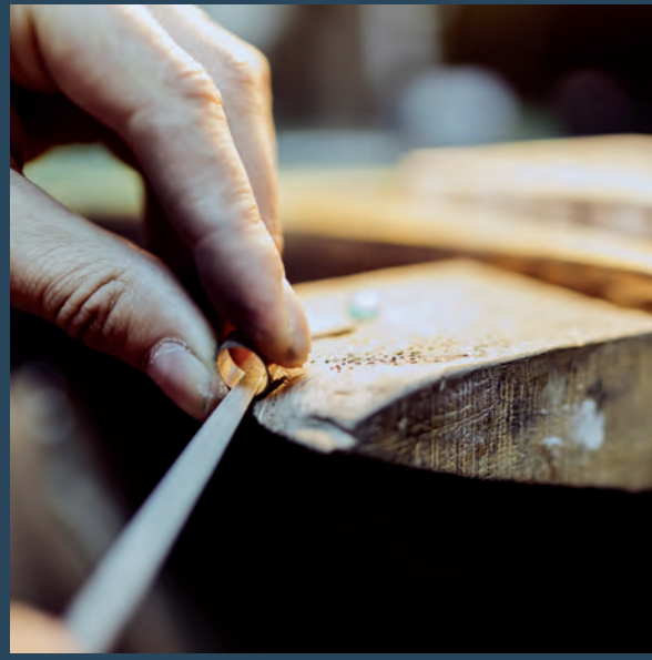
A goldsmith filing the inside of a ring with a special jewellery file
