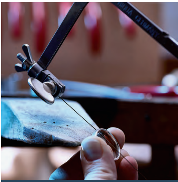
Jeweller's saw blade sawing open a ring - thanks to the tiniest saw teeth, hardly any valuable material is abraded in the process
